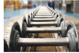
轮轴 Wheel Sets complete with Class E Wheel Bearing
